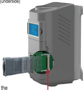
Anybus slot and 50-pin CompactFlash connector on the PCB of the host device
